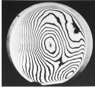
Fig. 4.1. Interference contours of silicon wafer surface deformation.
