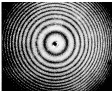
Fig. 3.12. Interference pattern of two specklegrams positioned one behind another.
