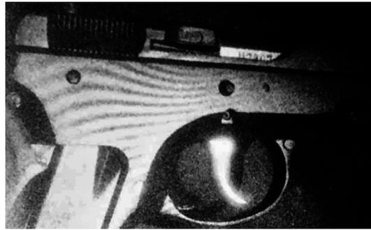
Fig. 2.1. Double-exposure Fresnel type holographic interferogram of the gun deformation between two subsequent shots. The interference fringes represent isolines of equal magnitude of deformations.
