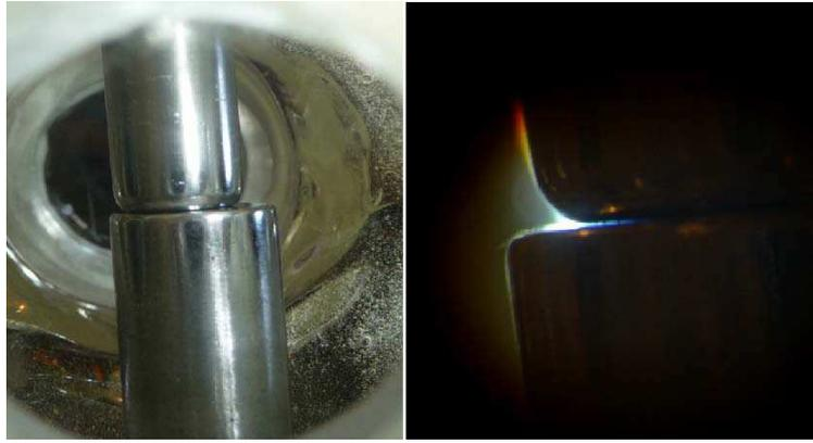
Fig. 18.6. Molybdenum electrodes with Bruce profile.
