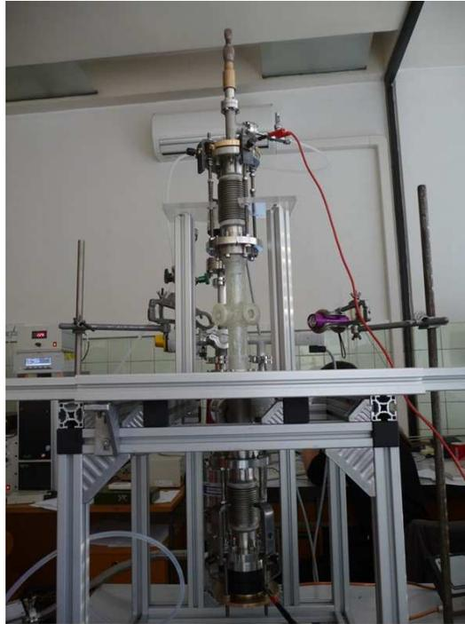
Fig. 18.1. Photograph of the apparatus used for the measurements of the DC breakdown voltage curves and volt-ampere characteristics at micrometer separations between two planar electrodes.
