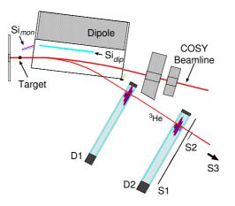
Fig. 1. Schematic view of the COSY-11 detection system [21].
