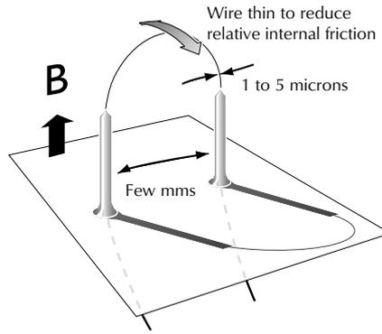
Fig. 1. A vibrating wire resonator.
