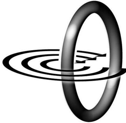
Fig. 7. A vortex ring moving in its own flow field.
