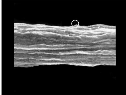
Fig. 3. A micrograph of the surface of a rough wire showing where vortices form at the excrescences.
