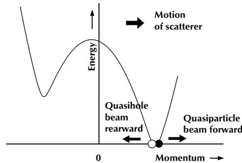
Fig. 2. The dispersion curve for superfluid  $^3\text{He}$  seen in a frame moving at the Landau critical velocity. The free production of quasiparticles and quasiholes occurs as the minimum in the dispersion curve touches zero energy.
