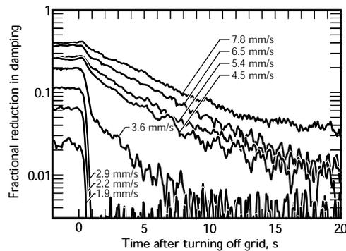
Fig. 5. The decay of vorticity after the grid is switched off, for a number of grid velocities.
