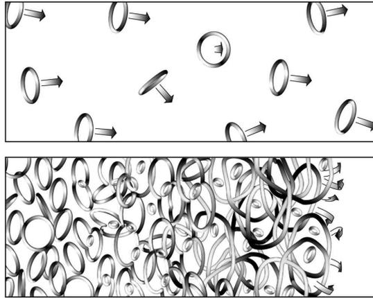
Fig. 8. Schematic view of the behaviour. At low grid velocities a tenuous gas of non-interacting vortex rings is formed as shown in the upper figure. However, in the lower figure, at higher grid velocities the ring density has become high enough that the vortex cores recombine forming a sluggish vortex tangle.
