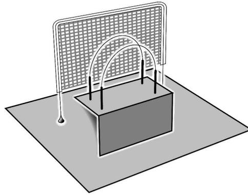
Fig. 4. A vibrating grid with the two detector wires in front.
