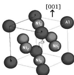
Fig. 1. The L1<sub>2</sub> structure of Ni<sub>3</sub>Al.
