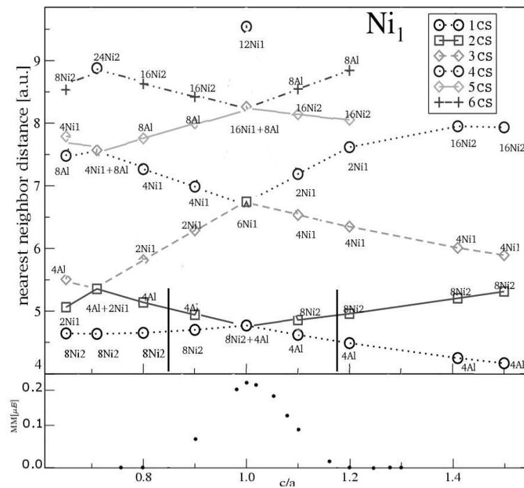
Fig. 4. The first six coordination spheres of  $Ni_1$  atom site of  $Ni_3Al$  with  $L1_2$  structure along the tetragonal deformation path. The lower panel of the figure shows the behavior of magnetic moment of  $Ni_1$  atom. The results for  $Ni_2$  atoms are similar.
