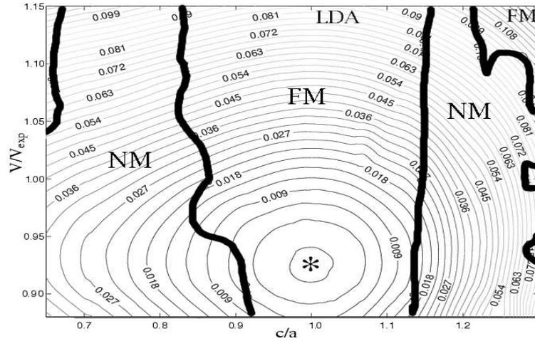
Fig. 2. The total energy (per formula unit) of Ni<sub>3</sub>Al [Ry] calculated within the LDA as a function of volume ( $V/V_{exp}$ ) and shape ( $c/a$ ) deformation. The asterisk denotes the ground-state of Ni<sub>3</sub>Al. For more details, see the text.
