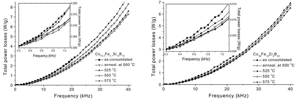
Fig. 1. Dependencies of total power losses on frequency for  $\text{Co}_{70.3}\text{Fe}_{4.7}\text{Si}_{10}\text{B}_{15}$  and  $\text{Co}_{56}\text{Fe}_{16}\text{Zr}_8\text{B}_{20}$  bulk samples.
