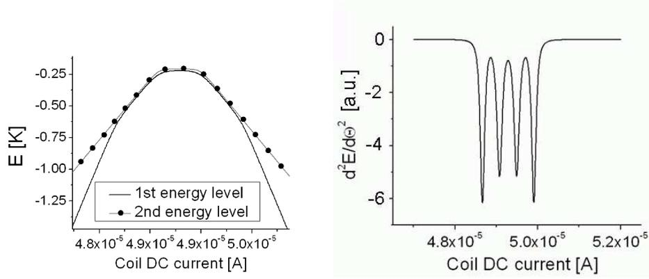
Fig. 2. (a) first two energy levels of a four-qubit system (on the left) calculated from Hamiltonian (1); (b) the second derivative of the first energy level of our four-qubit system (on the right). Coupling energies for all qubits are 0.1 K, tunneling amplitudes are 0.02 K.
