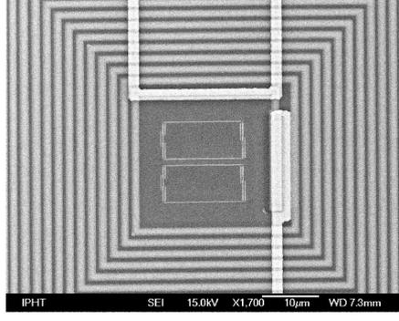
Fig. 1. Two superconducting flux qubits inside the coil of the resonant tank circuit. Using  $I_{dc2}$  (top wire) and  $dc$  current through the coil we are able to change biases of the individual qubits independently.
