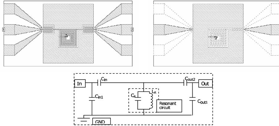
Fig. 4. Model of new high-frequency high-quality resonant tank circuit for frequencies above 1 GHz. Sonnet software two-layer model (the upper panels); schematic (the bottom panel).
