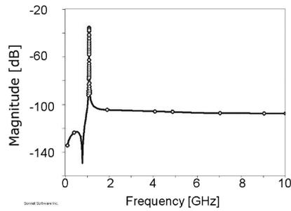
Fig. 5. Response function (S21 parameter) of the tank circuit. Quality factor  $Q \approx 10^4$ .
