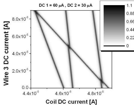
Fig. 3. The  $\tan(\theta)$  vs. external flux flow for four qubits. Using additional *dc* wires to change flux flow through one qubit, we are able to entangle one qubit with every other one;  $T = 50$  mK,  $J_{ij}/h = 410$  MHz,  $\Delta_i/h = 500$  MHz for all qubits.
