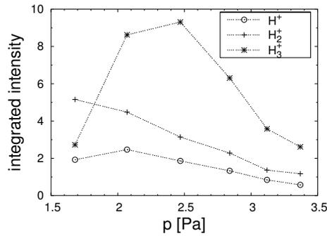
Fig. 6. Pressure dependence of the IED integrals measured at the glow region in the vertical distance from the powered electrode of 31 mm. The rf power was 30 W.
