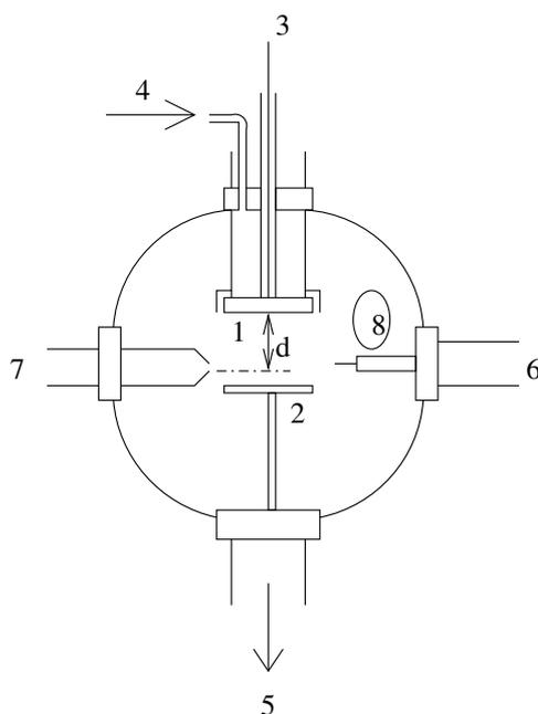
Fig. 1. The schema of the experimental apparatus: 1. rf electrode, 2. grounded electrode, 3. rf power input line, 4. feeding of gases, 5. towards vacuum pumps, 6. horizontally movable Langmuir probe, 7. PPM 421 devise, 8. quartz window for emission spectroscopy. Vertical distance between the rf electrode and extraction orifice of the PPM 421 is denoted  $d$ .
