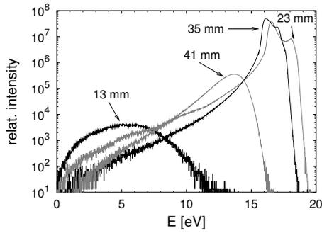
Fig. 2. IED of  $\text{H}_3^+$  in different vertical distances from the rf electrode for 2.5 Pa and 30 W.
