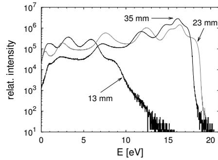
Fig. 3. IED of  $\text{H}_2^+$  in different vertical distances from the rf electrode for 2.5 Pa and 30 W.
