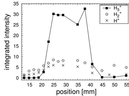
Fig. 5. Integrals of the IEDs of  $\text{H}^+$ ,  $\text{H}_2^+$  and  $\text{H}_3^+$  in different vertical distances from the rf electrode. 40 mm is the position of the grounded electrode.
