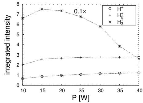
Fig. 7. Dependences of the IED integrals on rf power at 1.65 Pa. In order to compare all three ions in the same graph the values for  $H_3^+$  were  $10\times$  decreased. The  $H^+$  IED was measured with different voltage on the multiplier.
