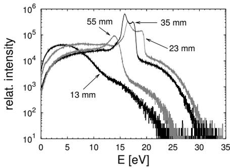
Fig. 4. IED of  $\text{H}^+$  in different vertical distances from the rf electrode for 2.5 Pa and 30 W.
