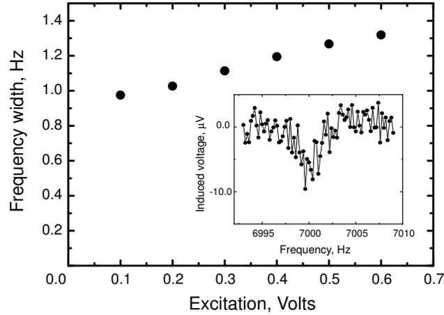
Fig. 3. The dependence of  $\Delta f_2$  on the excitation voltage. measured at  $T = 1$  mK and  $B = 15$  mT. Inset: the presence of the second harmonics in oscillations of the vibrating wire documents the nonlinear properties of the resonator.
