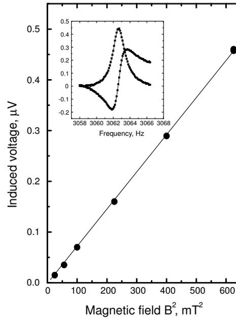
Fig. 2. The dependence of the induced voltage by the vibrating wire on magnetic field. Inset shows typical induced resonance signals measured during the frequency sweep.
