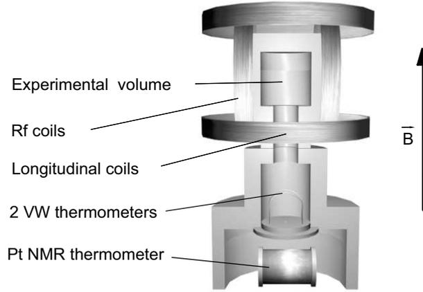
Fig. 1. The 3-D cross section of the experimental cell.
