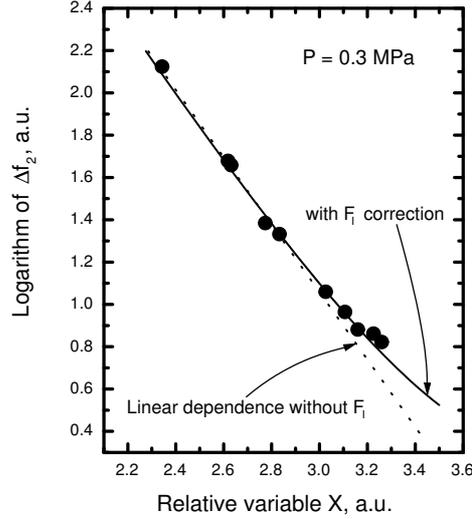
Fig. 5. The dependence of  $\Delta f_2$  on temperature with and without correction of the intrinsic damping of the vibrating wire.
