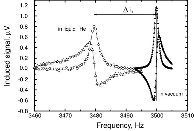
Fig. 4. Typical induced signal from vibrating wire measured in vacuum and liquid  $^3\text{He}$ . The frequency shift from the resonance frequency in vacuum and increase of damping due to presence of the liquid is clearly seen.
