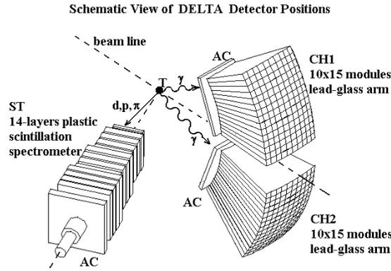
Fig. 13. A schematic view of the DELTA-2 setup. T – polarized proton target PPT; CH1, CH2 – two arms of the Čerenkov lead-glass spectrometer for two gammas after neutral meson decay measurements, ST – 14-layer fiber-optic scintillation telescope for multi- $\Delta E$  measurements of charged particles, AC – anticoincidence detectors.
