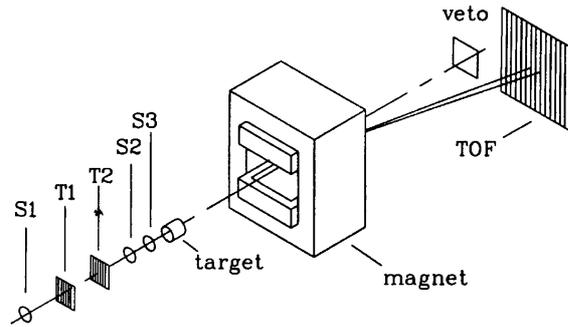
Fig. 21. The scheme of the SCAN-2 setup.
