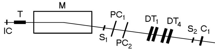
Fig. 9. The scheme of the STRELA setup which was exposed in the June 2003 Nuclotron run.
