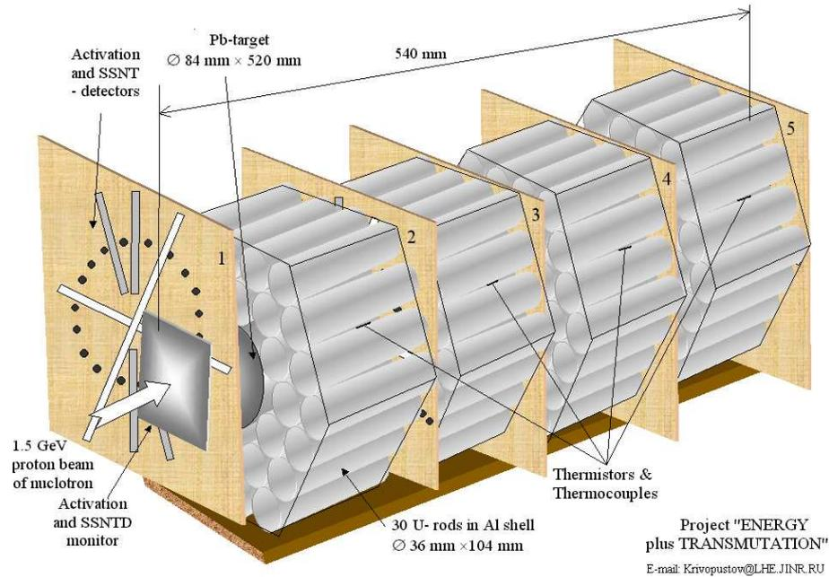
Fig. 29. The scheme view of the Energy + Transmutation setup.
