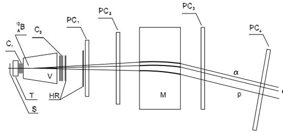
Fig. 27. SPHERE spectrometer modified to investigate the nonmesonic decay of  $^{10}_{\Lambda}\text{B}$  produced in the Nuclotron carbon beam. S – the beam control counters, T – the target,  $C_{1,2}$  – the trigger Čerenkov counters, V – vacuum decay volume, HR – the high resolution detectors, M – the magnet,  $PC_{1-4}$  – the proportional chambers.
