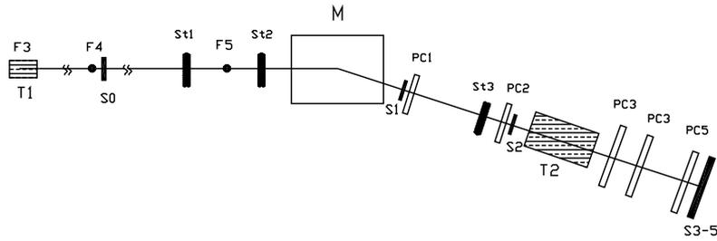
Fig. 12. The scheme of the setup.  $S_i$  – scintillation counters,  $PC_i$  – proportional chambers,  $St_i$  – straws,  $M$  – magnet,  $T_i$  – targets.
