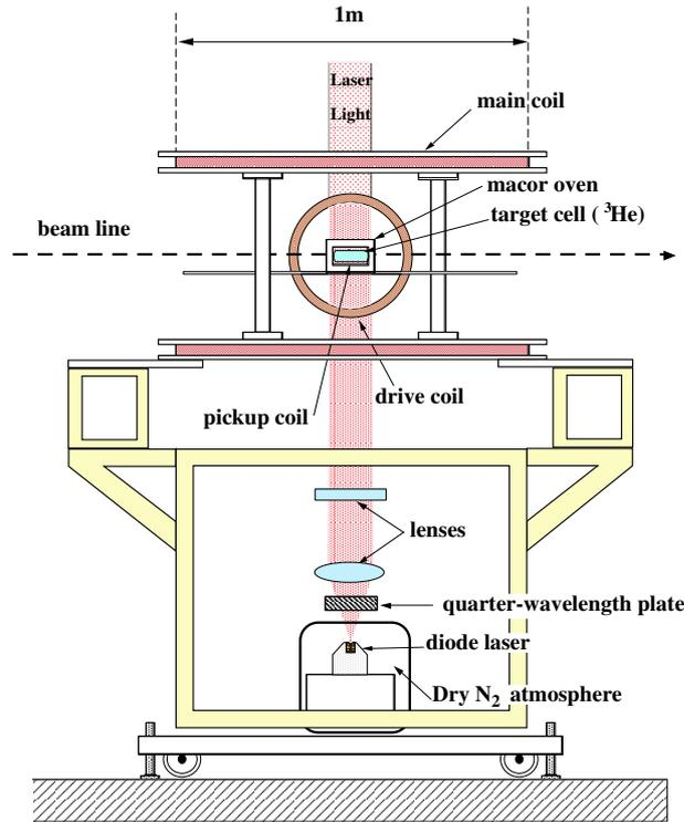
Fig. 17. Schematic view of the polarized  $^3\text{He}$  target.
