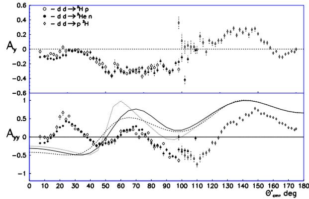
Fig. 16. The angular dependence of the vector and tensor analyzing powers in the center-of-mass frame measured at 270 MeV. The solid, dot-dashed and long-dashed curves are the results of the ONE calculations made by [22] using different  ${}^3\text{He}$  wave functions.
