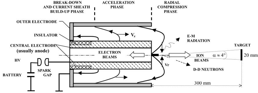
Fig. 1. Scheme of dense plasma-focus processes and target location
