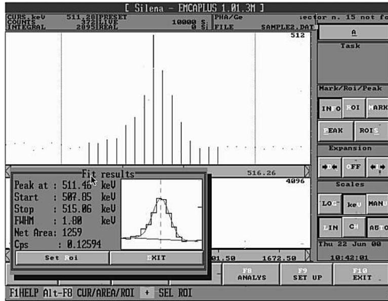
Fig. 3. The spectrum of gamma quanta emitted from activated carbon target. Photo peak with energy 511 keV has been expanded and analyzed in the left down corner.
