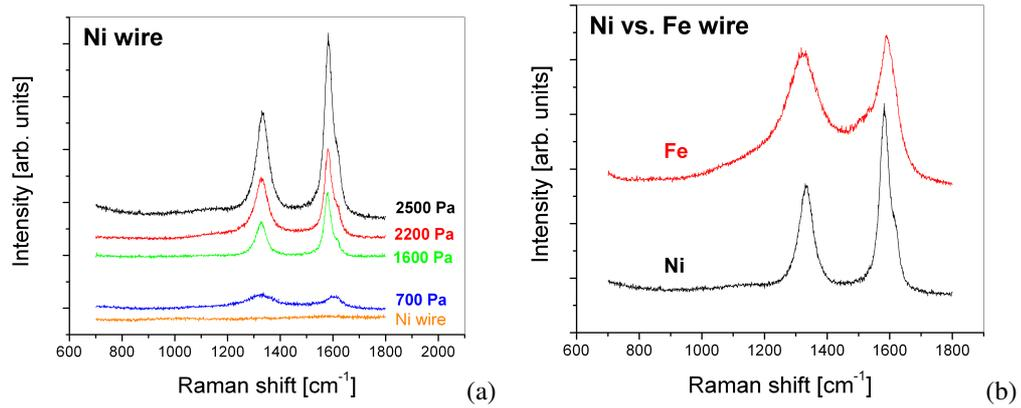
Fig. 1. Raman spectra of samples (a) Ni wire in dependence on pressure, and (b) Ni and Fe wires.
