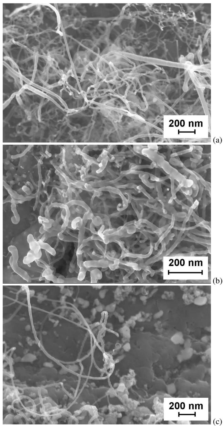
Fig. 3. SEM micrographs of carbon nanotubes (a) grown on Ni wire at 2500 Pa, (b) grown on Fe wire at 2500 Pa, (c) grown on Ni wires at 1600 Pa.
