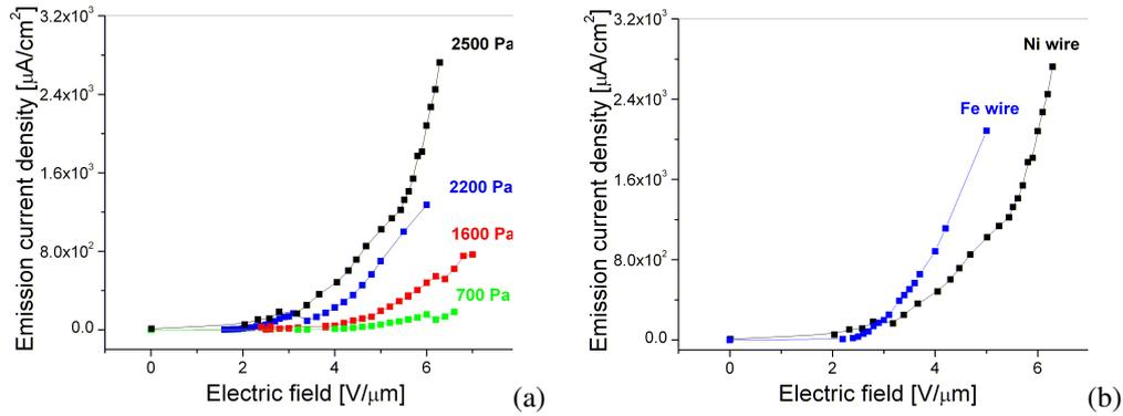
Fig. 2. Cold electron emission measurements of (a) nanotubes deposited on Ni at different pressures, and (b) comparison of cold electron emission of nanotubes grown on Ni and Fe wires.
