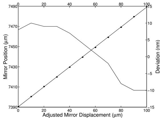
Fig. 4. The mirror positions determined from the processed spectral interferograms as a function of the adjusted mirror displacement (points) and the corresponding deviations: the first fused-silica sample.
