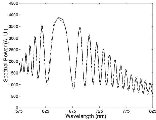
Fig. 3. Example of the recorded spectral interferogram compared with theory (dashed line): the first fused-silica sample.
