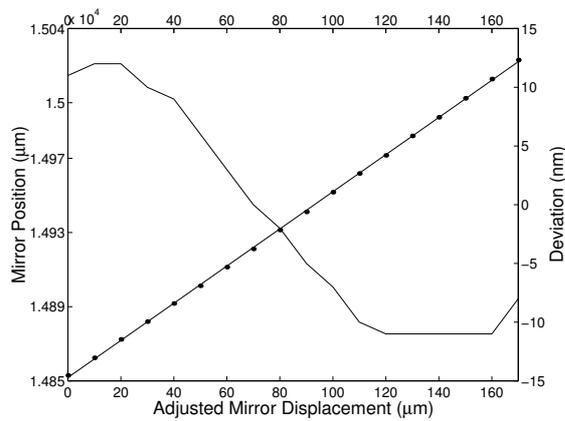
Fig. 6. The mirror positions determined from the processed spectral interferograms as a function of the adjusted mirror displacement (points) and the corresponding deviations: the second fused-silica sample.
