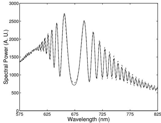
Fig. 5. Example of the recorded spectral interferogram compared with theory (dashed line): the second fused-silica sample.
