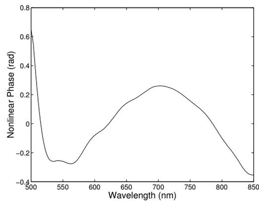
Fig. 2. Measured nonlinear phase as a function of the wavelength.
