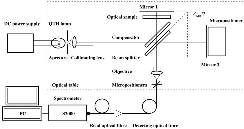
Fig. 1. Experimental set-up with a dispersive Michelson interferometer to measure distances and displacements of the interferometer mirror.
