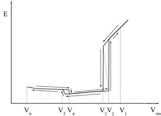
Fig. 2. Dependence of  $E$  versus  $V_{\text{rms}}$  characteristic of the RF plasmoid
