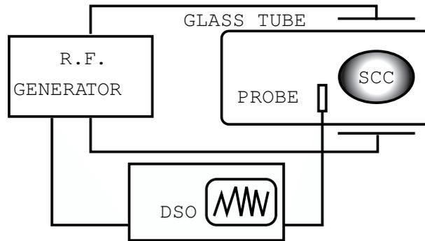
Fig. 1. Experimental device
