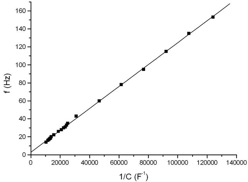
Fig. 4. The linear dependence between the oscillation frequency and the inverse of the capacitance.
