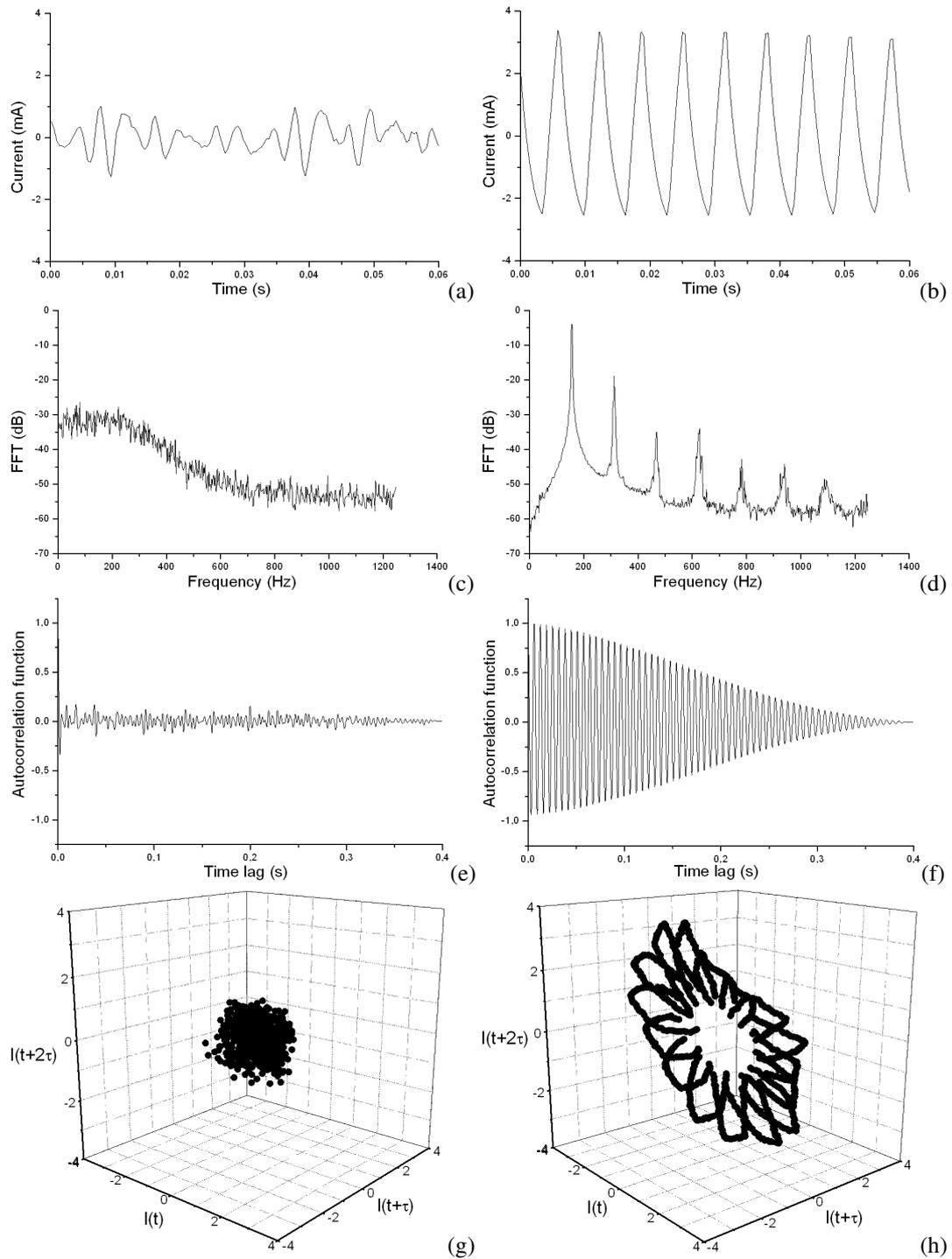
Fig. 3. The time series, the FFT, the autocorrelation function, and the 3D Poincaré map through the reconstructed space of the current oscillations, respectively, before (left column) and after (right column) the insertion of the capacitor (we find the delay time  $\tau = 1.6$  ms).
