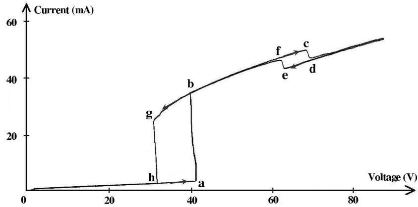
Fig. 2. Static  $I - V$  characteristic obtained in a DP-machine plasma.
