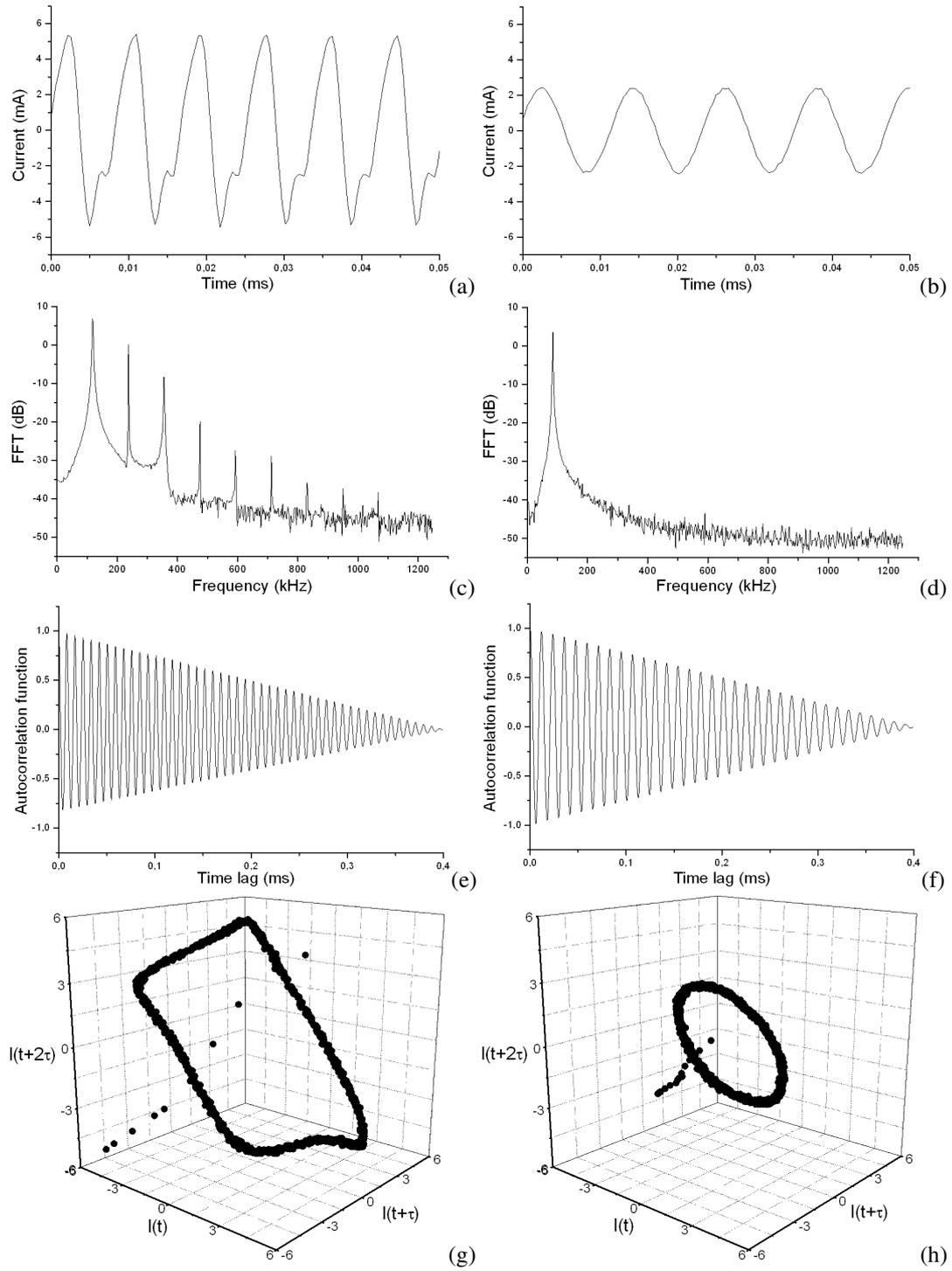
Fig. 5. The time series, the FFT, the autocorrelation function, and the 3D Poincaré map through the reconstructed space of the current oscillations, respectively, before (left column) and after (right column) the connection of the coil (we find the delay time  $\tau = 2.4 \mu\text{s}$ ).
