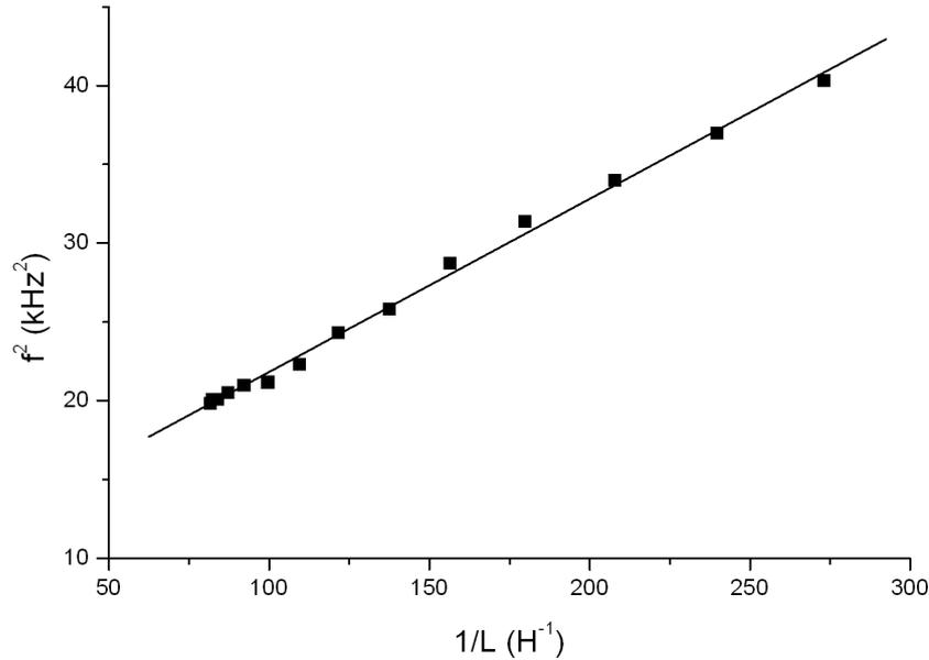
Fig. 6. The linear dependence between the square of the oscillation frequency and the inverse of the inductance (according to the Thomson formula).
