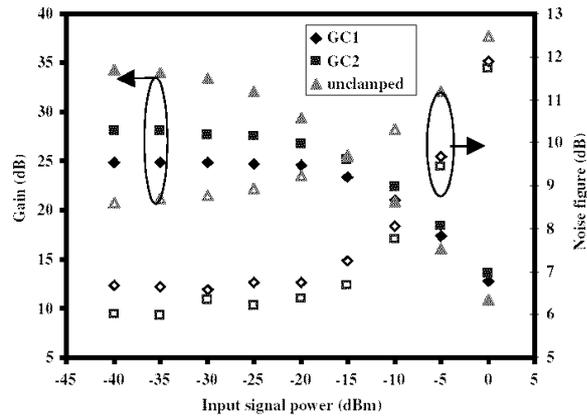
Fig. 7. Gain (closed) and noise figure (clear) as functions of input signal power for double-pass system.
