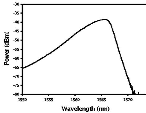
Fig. 2. Forward ASE at the L-port of C/L-band WDM with open-ring.
