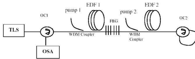
Fig. 5. Configuration of the proposed gain clamped L-band EDFA in double-pass system
