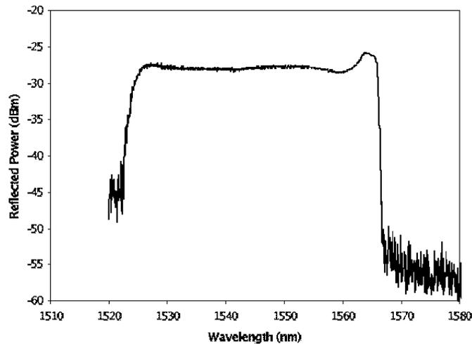
Fig. 6. Reflection characteristics of the broadband FBG
