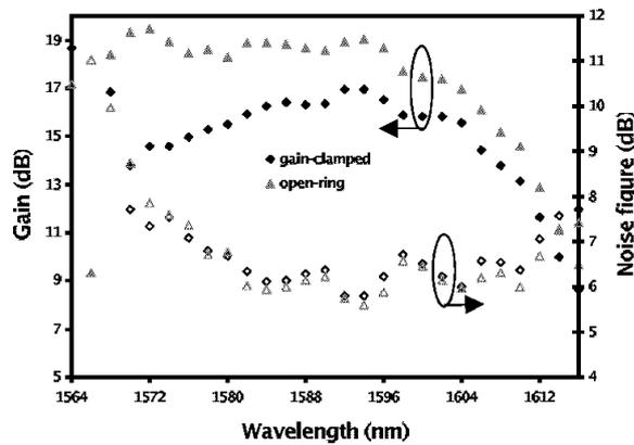
Fig. 4. Gain and noise figure as functions of input signal wavelength for single-pass system.
