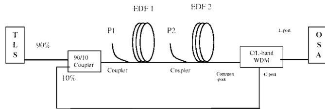
Fig. 1. Configuration of the proposed gain clamped L-band EDFA in single-pass system.
