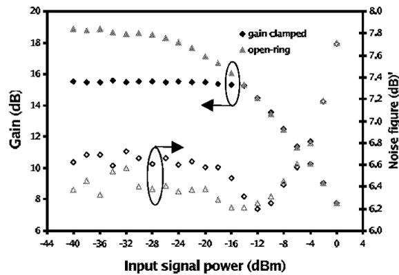
Fig. 3. Gain and noise figure against input signal power for single-pass system.
