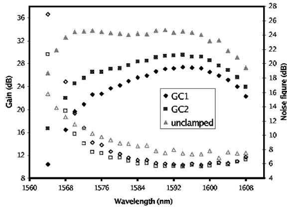
Fig. 8. Gain (closed) and noise figure (clear) as functions of input signal wavelength for double-pass system.
