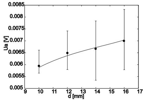
Fig. 8. Dependence of amplitude of pulses on distance of plate electrode for multi-needle. Supply voltage 6 kV.
