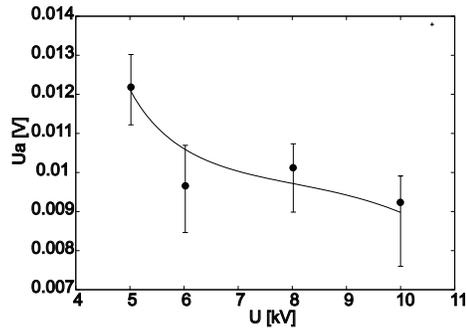
Fig. 6. Dependence of amplitude of pulses on supply voltage. Distance of plate electrode 10 mm. Radius of tip  $50 \mu\text{m}$ .
