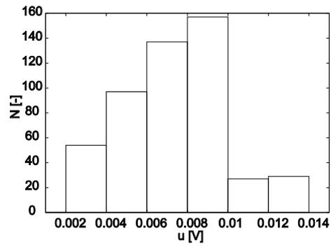
Fig. 10. Histogram of amplitude of corona discharge current for discharge burning on seven steel needles with interelectrode distance 2.5 mm a distance of plate electrode 10 mm. Voltage 10 kV.
