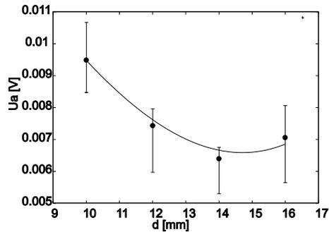
Fig. 4. Dependence of amplitude of pulses on distance of plate electrode for 6 kV. Radius of tip 50 μm.
