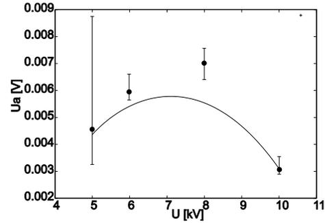
Fig. 9. Dependence of amplitude of pulses on supply voltage. Distance of plate electrode 10 mm.
