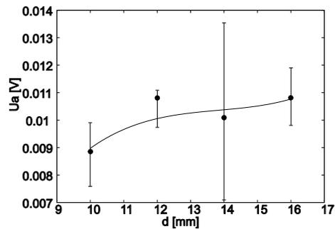
Fig. 5. Dependence of amplitude of pulses on distance of plate electrode for 10 kV. Radius of tip 50 μm.
