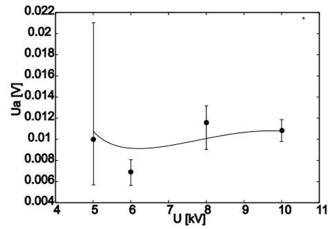
Fig. 7. Dependence of amplitude of pulse on supply voltage. Distance of plate electrode 16 mm. Radius of tip  $50 \mu\text{m}$ .
