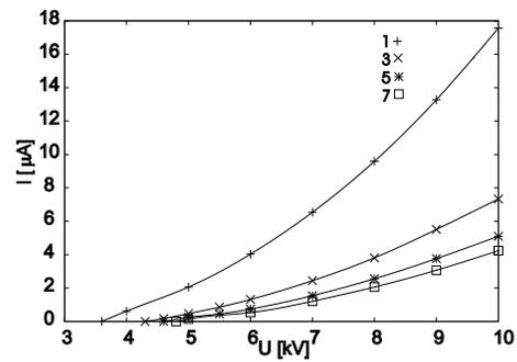
Fig. 3. VA characteristics for various multi-needle configurations. Normalised current to one needle. Number of needles: 1, 3, 5 and 7. Interelectrode distance 2.5 mm. Distance of plane electrode 12 mm. Radius of tip 50 μm.
