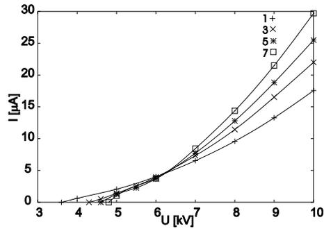
Fig. 2. VA characteristics for various multi-needle configurations. Number of needles: 1, 3, 5 and 7. Interelectrode distance 2.5 mm. Distance of plane electrode 12 mm. Radius of tip 50 μm.
