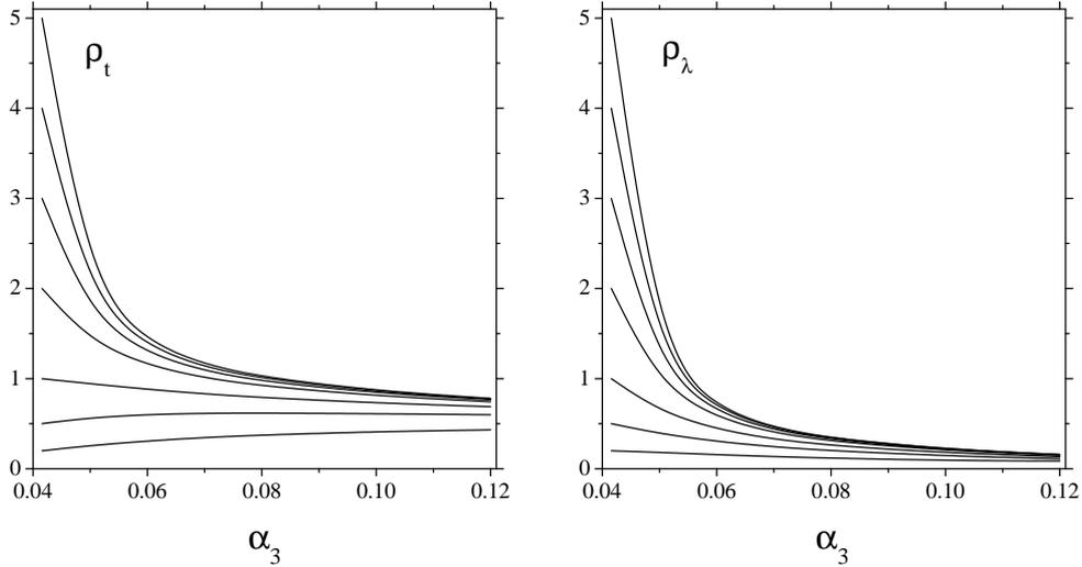
Fig. 1. The IRQFP behavior for  $\rho_i = Y_i/\tilde{\alpha}_3, i = t, \lambda$  as functions of  $\alpha_3$ . The value  $\alpha_3 \approx 0.042$  corresponds to the GUT scale, and the value  $\alpha_3 \approx 0.12$  corresponds to the electroweak scale.
