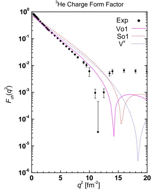
Fig. 2.  $^3\text{He}$  charge form factors using Gaussian shape potentials. Experimental points are taken from Ref. [4].
