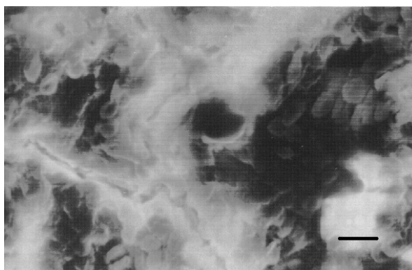
Fig. 5. Particles of inorganic material are visible. Seize and shape of particles are various. SEM micrograph, line size is 10 \mu\text{m} .
