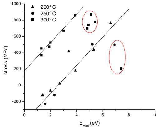
Fig. 5. Internal stress as function of  $E_{\max}$  in the pressure series at 50 MHz. Plotted are the results for three different temperatures. Lines are guides to the eye.
