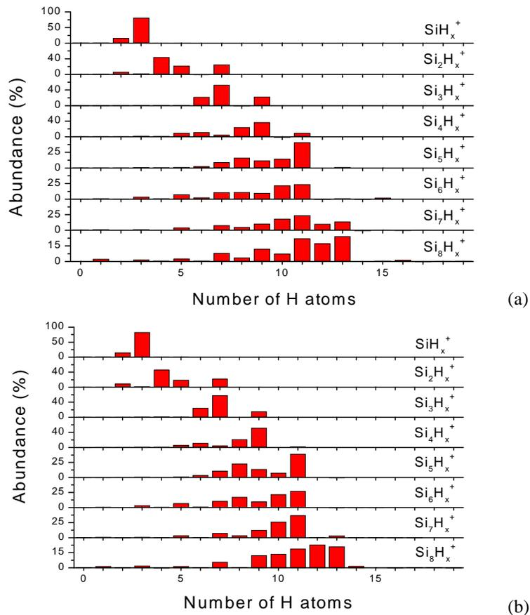
Fig. 7. (a) The relative abundance of ions with different amount of H atoms for the different Si numbers at (a) 12 Pa, and (b) 50 Pa.
