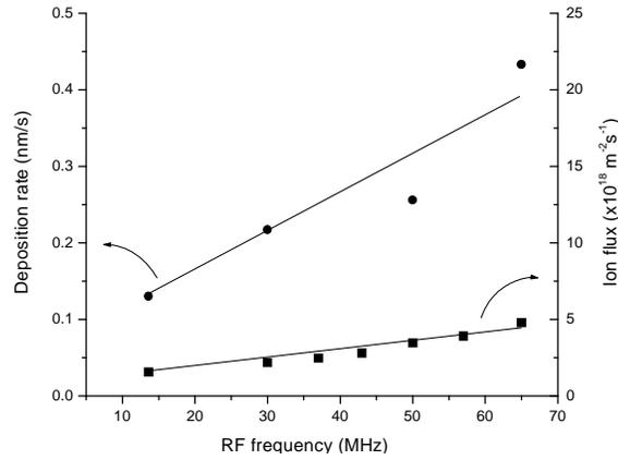
Fig. 2. The growth rate  $r_d$  and ion flux as function of the RF frequency. The right hand axis is scaled to the left hand side axis as is explained in the text. Lines are guides to the eye.
