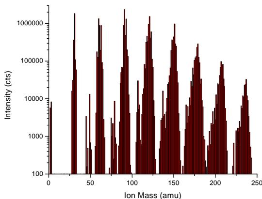
Fig. 6. Ion mass spectrum, corrected for the mass transmission function of the mass spectrometer. The plasma conditions are 10 W RF power, RF frequency of 050 MHz, process pressure of 12 Pa, and flows of 30 sccm  $\text{SiH}_4$  and 30 sccm  $\text{H}_2$ .
