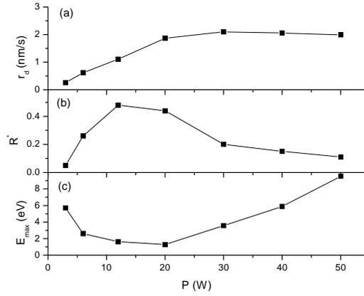
Fig. 3. The growth rate  $r_d$  (a), the microstructure parameter  $R^*$  (b), and the kinetic ion energy per deposited atom  $E_{\max}$  (c) as function of power in a silane-argon plasma.
