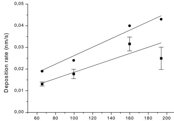
Fig. 9. The growth rate and the growth rate due to the ions as function of process pressure. The circles represent the total growth rate, the squares the growth rate due to the ions. Under these conditions microcrystalline silicon is formed.
