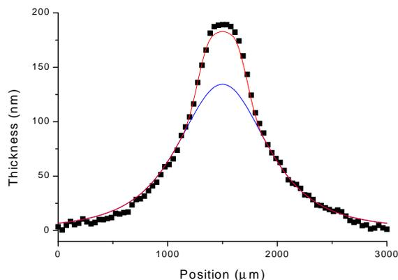
Fig. 8. The deposition profile behind an circular orifice. The wings are completely due to deposition of radicals, while the central part has also a contribution of ions. The surface reaction probability of the radicals is 0.42 and the ion contribution is 4%. The solid lines are the fitted radical (lower curve) and radical plus ion profile (upper curve in central part). For a detailed description of the method see Ref. [3, 4].
