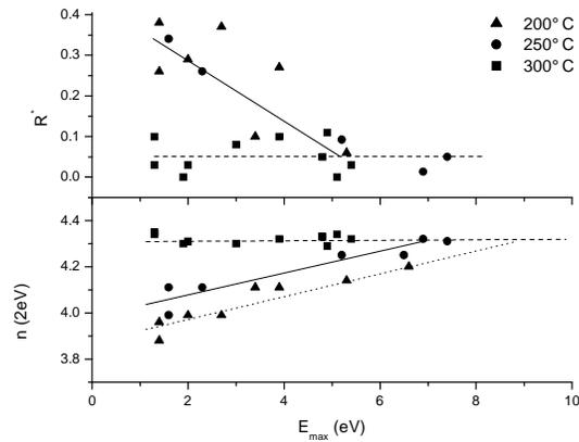
Fig. 4. Material properties as function of  $E_{\max}$  at three substrate temperatures: (a) the microstructure parameter  $R^*$  and (b) the refractive index  $n$  at a photon energy of 2.0 eV.
