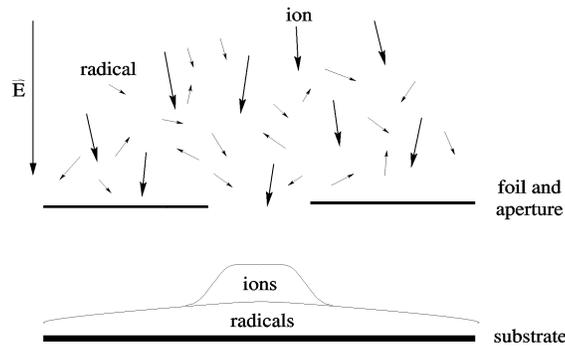
Fig. 1. Schematic diagram of the deposition profile of both radicals and ions behind an aperture.
