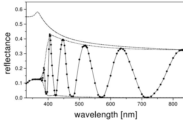
Fig. 9. ZnO/Si reflectance (solid line), the envelopes (dashed), bare Si reflectance (dashed–dotted line).
