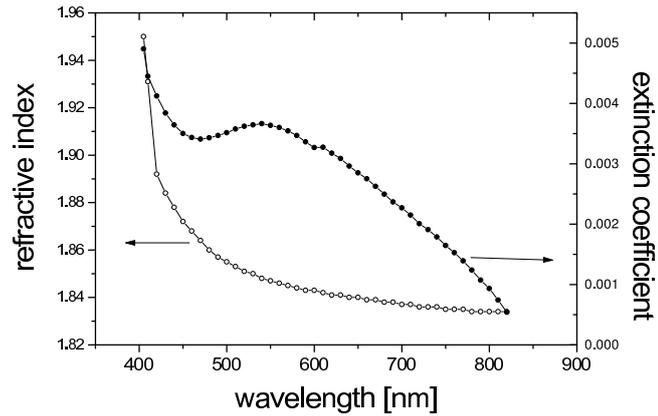
Fig. 11. Optical constants of ZnO thin film.
