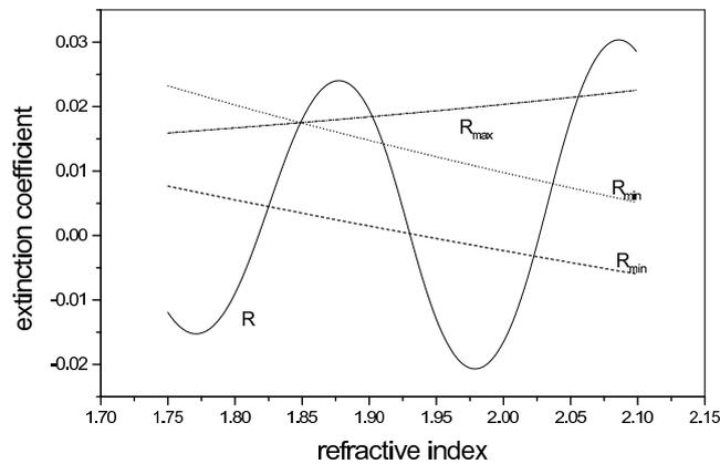
Fig. 4. Iso reflectance contours for the hypothetical film at the wavelength 500 nm.
