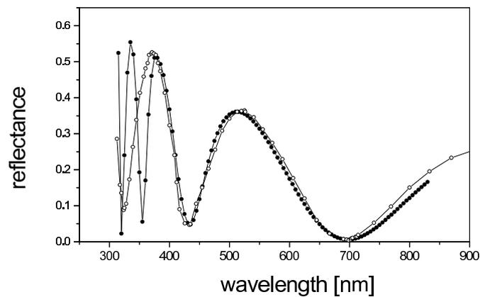
Fig. 10.  $Y_2O_3/Si$  reflectance, open points – experimental values, solid points – retrieved reflectance.
