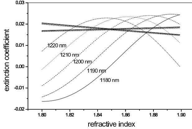
Fig. 5. Iso reflectance contours for the changing thickness, the intersection only for  $d = 1200$  nm.
