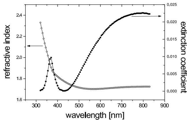
Fig. 12. Optical constants of  $Y_2O_3$  thin film.
