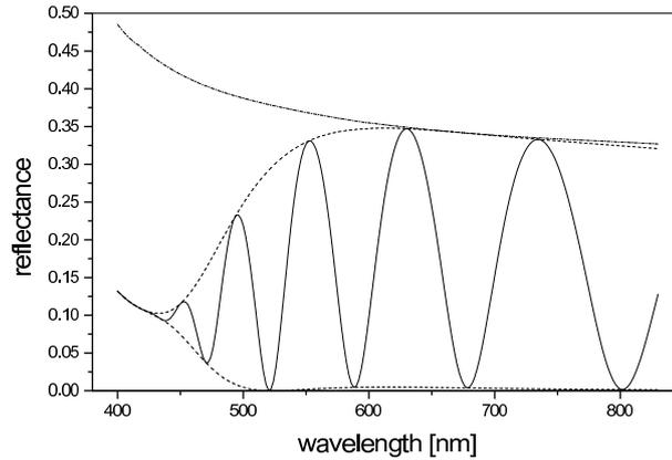
Fig. 1. Reflectance of the hypothetical film (solid curve), of the envelopes (dashed curves), of the Si substrate (dashed–dotted curve).
