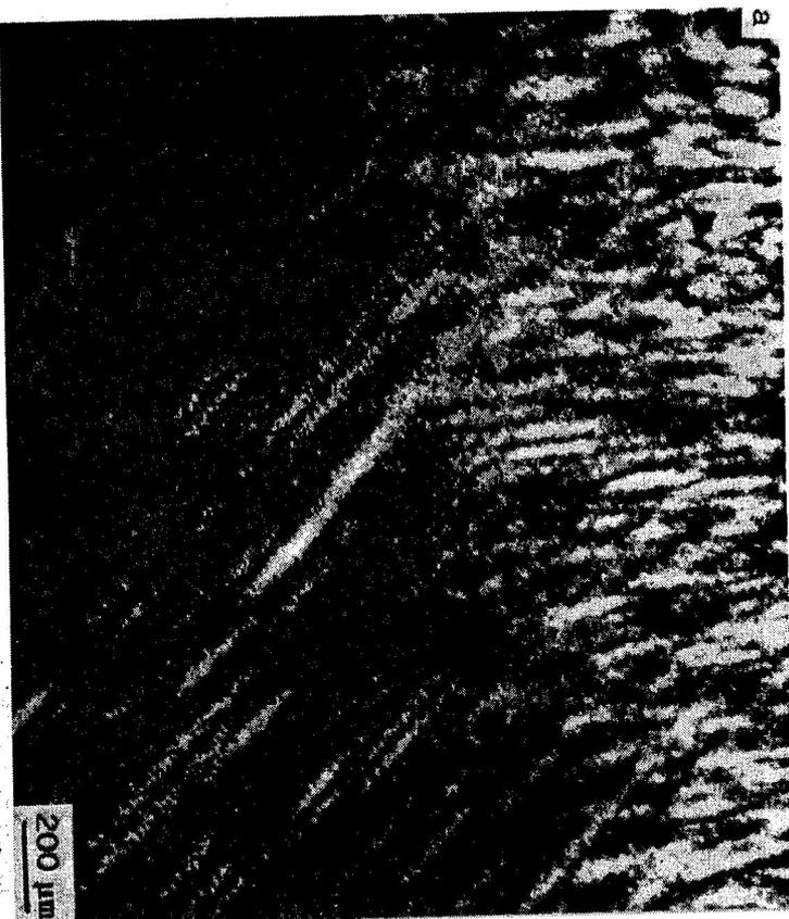
Fig. 3. Slip bands observed on the surface of aluminium: a) and b) parallel slip bands ( $\epsilon = 8\%$ ); slip direction make the angle of  $45^\circ$  with the tensor axis.
