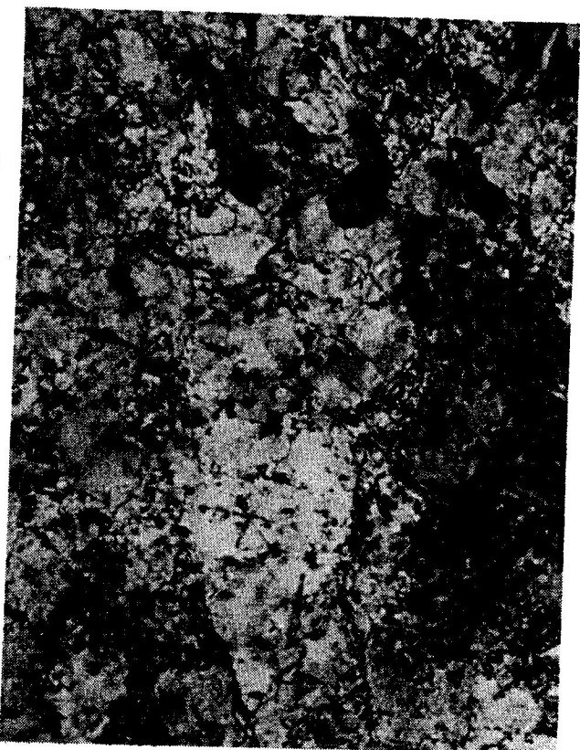
Fig. 3. Dislocation configuration at 8% strain, V-steel.
