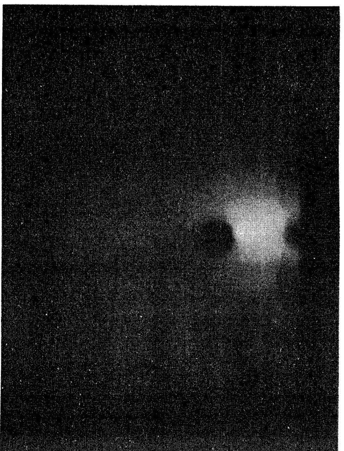
Fig. 3. Photograph of the electron beam from cathode into central electrode ( I_k = 300 mA; U_k = 4.7 kV; p = 13.7 Pa).
