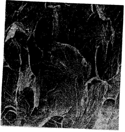
Fig. 2. Morphology of the transcrystalline cleavage fracture of Fe-3% Si alloy (100x).
