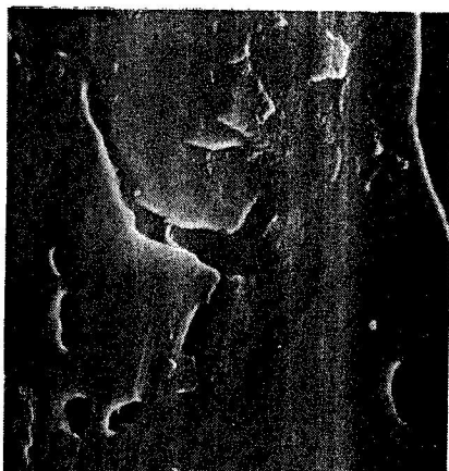
Fig. 10. Filamentary character of over-ohmic current transport in pictures of the sample's vertical cross-section. Diameter of melted channel is about 5 \mu\text{m} . Enlargement 680 \times .
